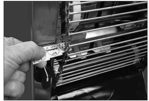
Figure 10. Measuring Conveyor Belt Chain
