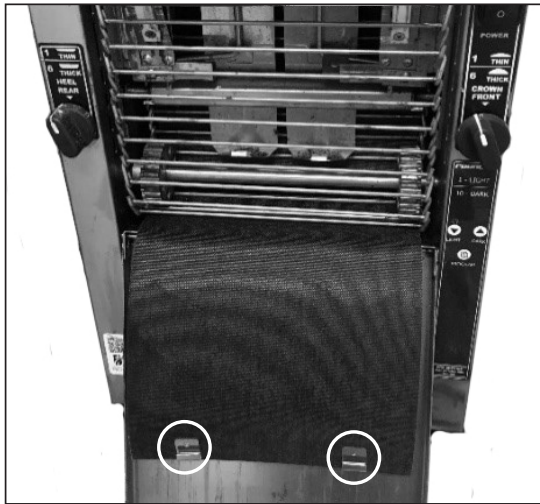
Figure 6. Replacing Belt Wraps
