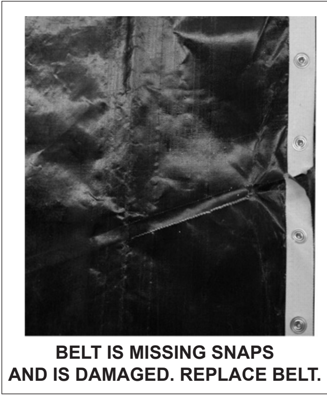
Figure 11. Example of Damaged Belt
