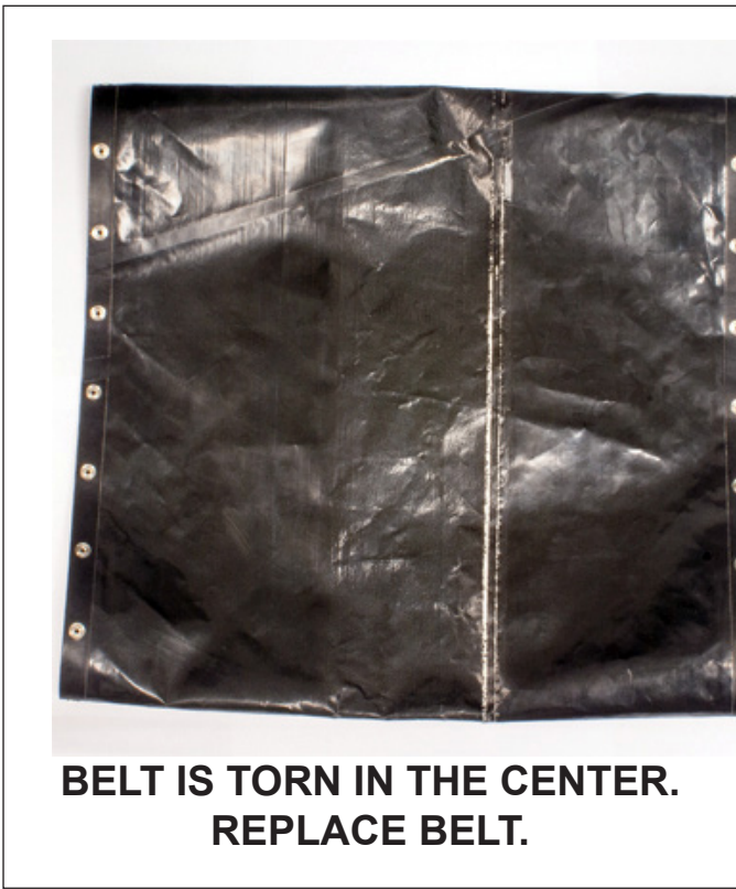
Figure 12. Example of Damaged Belt
